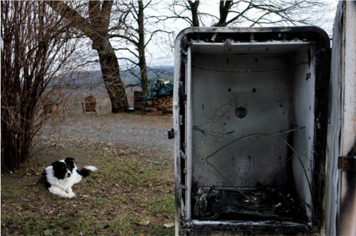
A try at running a homemade smoker didn't go well at Fat Rooster Farm. A hot plate in the old refrigerator caught fire, burning up the meat and everything else.
