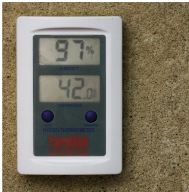
RIGHT: A hydro-thermometer measures temperature and humidity in the root cellar at Fat Rooster Farm.
